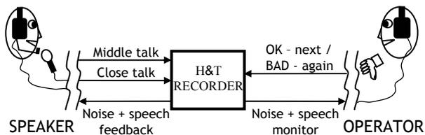
Figure 1: Recording setup
